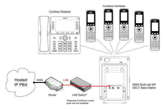
Figure 1. M500 Installation Example (single cell configuration)
