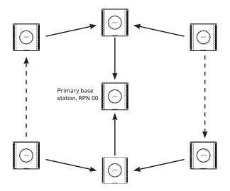
**Continuous line**: Shows the primary sync paths, with the relevant base stations chained in the multicell network. **Dotted line**: Alternative sync paths if base station within range.
