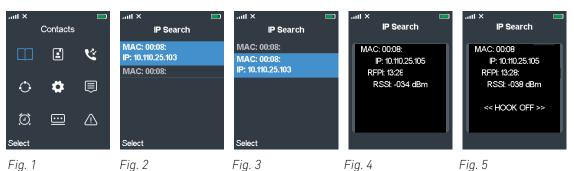
4. If necessary, scroll to the MAC address of your base station. The selected item is highlighted in blue and expands to also show the IP address of the base station (Fig. 2 and 3).
